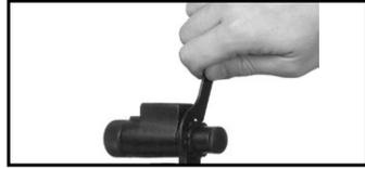
You could change the IR control panel fitting your needs. The screw-tool included into the set should be used for weakening the fixing screw located on the IR. Rotate the IR placing at in the most convenient position. Tighten the screw with the screw-tool to fix the new position.
