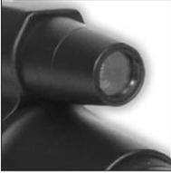
Infra-red illuminators, or IR illuminators, are common to night vision. The IR light greatly enhances the performance of the Viper while remaining almost totally invisible to the naked eye. The IR illuminator on the Viper is located underneath the front lens, next to the battery compartment.
