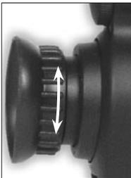
To focus the Viper, first you will need to adjust the diopter. Simply turn the diopter clockwise until it stops. Then, while looking through the diopter at an object, slowly turn the diopter back counter clockwise until the grain in the image is sharp.
