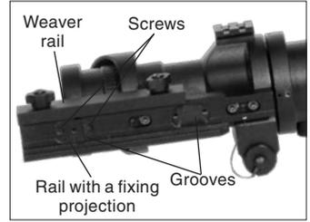
**NOTE:** If the rail is not taken out easily, screw up tight one of screws into the threaded aperture in the middle of a fixing projection of the rail. Continue rotation of the screw. Thus the screw will push out a rail from a groove.
